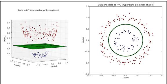
Figure 6: (Left) The decision boundary  $\vec{w}$  shown to be linear in  $\mathbb{R}^3$ . (Right) The decision boundary  $\vec{w}$ , when transformed back to  $\mathbb{R}^2$ , is nonlinear.
