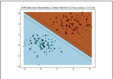
Figure 2: The Decision Boundary of a Linear SVM on a linearly-separable dataset. The solid line is the boundary. The SVM is trained on 75% of the dataset, and evaluated on the remaining 25%. Circled data points are from the test set.
