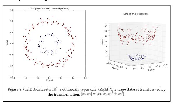
Let's think outside the box for a moment. Consider the linearly nonseparable dataset in Figure 5 (left), with its two concentric rings. Imagine that this dataset is merely a 2-D version of the 'true' dataset that lives in  $\mathbb{R}^3$ , Figure 5 (right). The  $\mathbb{R}^3$  dataset is easily linearly separable by a hyperplane. Thus, provided that we work in this  $\mathbb{R}^3$  space, we can train a linear SVM classifier that successfully finds a good decision boundary.
